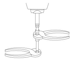
! CAUTION •Hold the spindle in place while doing this procedure, or internal instrument failure may result. Use a rag to protect the spindle's surface. The spindle may not move smoothly if scratched.
